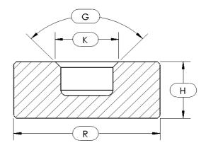
\*All Chamfer Masters come standard with flat lapped bottom
